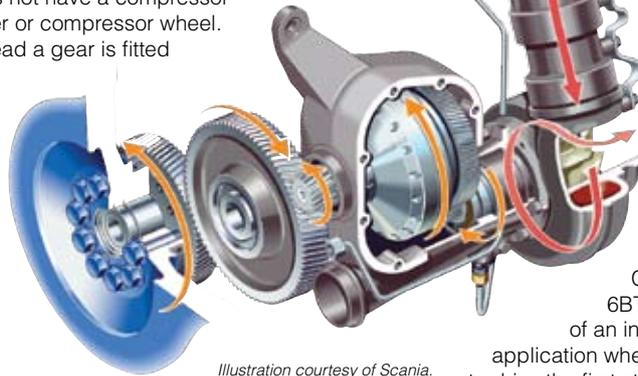
to the power turbine shaft. To assist the Power Turbine, a smaller turbine size is selected for the conventional turbocharger.
