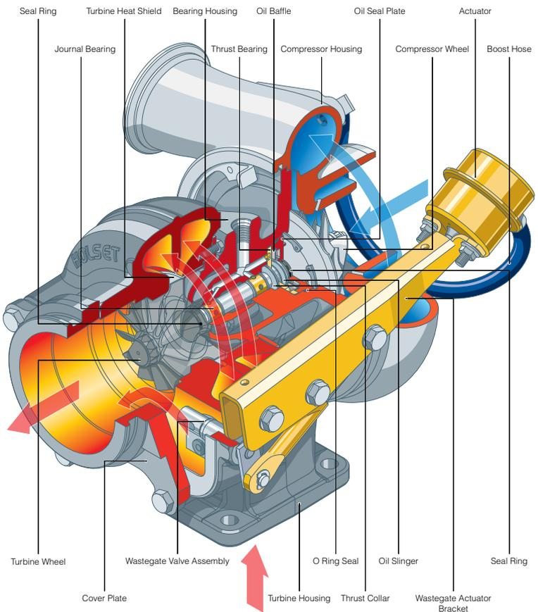
The **journal bearings** are a free floating rotational type. To perform correctly, the journal bearings should float between a film of oil. The bearing clearances are very small, less than the width of a human hair. Dirty oil or blockages in the oil supply holes can cause serious damage to the turbocharger.
